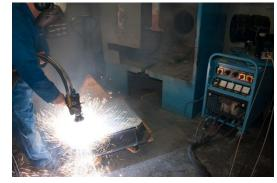
aluminium before being coated with 300 microns of 28E. This is the standard specification for external applications, offering unsurpassed corrosion resistance and durable grip to ferrous items.
